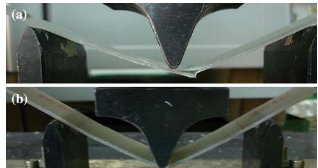
Fig. 13 The failure shapes of the wrinkled models
